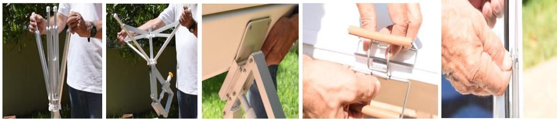
To place the tracking stand, first open slightly the two opposite legs and then the other two, to their limit. Then place it on a stable ground. Lift Sunchef and slide the aluminum plate which is found at its bottom, inside the corresponding socket on the top of the tracking base.
