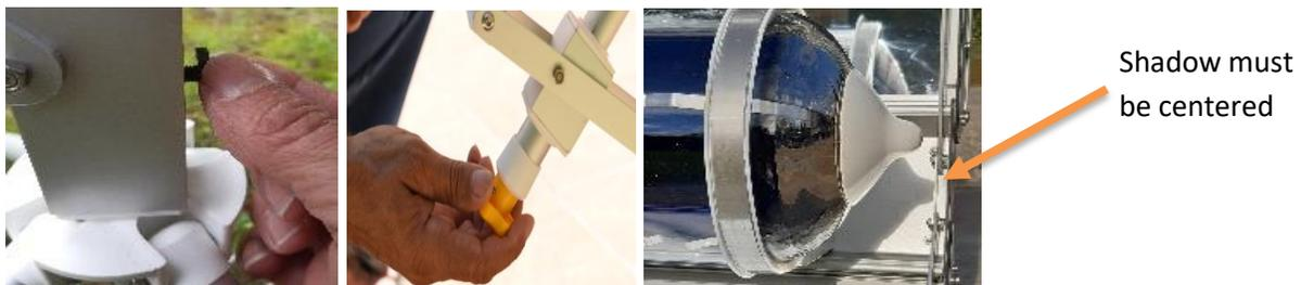
You can track the sun horizontally by turning Sunchef left or right accordingly. For the vertical tracking use the orange knob. Sunchef is at the right place when the shade of the end side of the glass tube is in the middle of the base of Sunchef and tangent to its vertical side.
