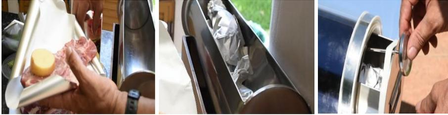
The inside of the borosilicate glass tube is protected from vapor and water from the food by a stainless steel tube. The food is placed in the special round shaped stainless steel pan and is then inserted into the stainless steel tube. You have the choice to use special oil paper and then aluminum foil to wrap the food when needed to limit the high temperatures and avoid the pyrolysis of the fat in the food, especially meat.
