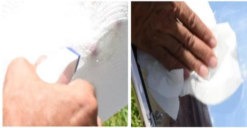
To clean the mirrors when dusty, always use wet kitchen paper with alcohol or glass cleaner. Never clean the glass tube when hot, only when it is at room temperature.
