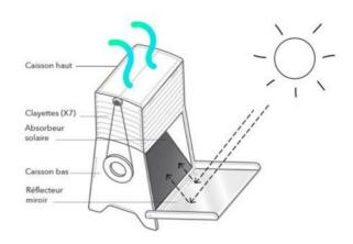
Modular, with 7 interchangeable shelves (higher, lower) for each type of food, OMY uses solar energy. The mirror reflector with adjustable inclination is positioned at the bottom of the dryer to accelerate the radiation which is directed towards the black sheet "the solar absorber", located inside the drying box. The black plate absorbs the sun's radiation and converts it into heat.
